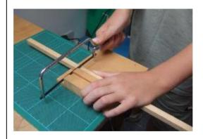
4. Along your pencil line, make a starter cut by pulling the saw back its whole length.
