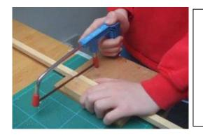
3. Keeping the saw straight, move it back and forth until it cuts all the way through the wood.
